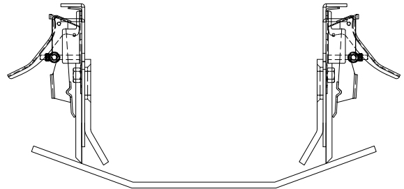
ASGCO straight Dura-Seal ORG Skirting With Double Handle Clamps, and angled wear liners.
