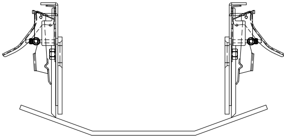
ASGCO straight Dura-Seal ORG Skirting With Double Handle Clamps, and straight wear liners.
